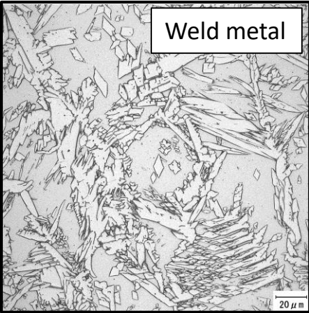
Photo. GMAW welded joint of UNS S82551 (OD273.1mm x WT14.3mm )
